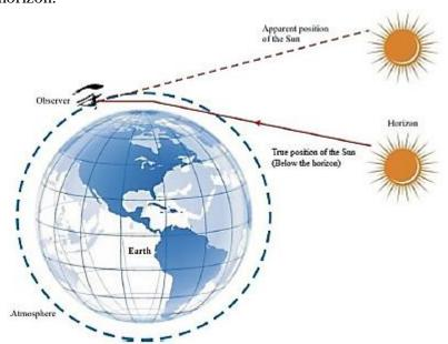
The increased atmospheric refraction of sunlight occurs also at sunset. In this case, the observer on the Earth continues to see the setting Sun for two minutes after the Sun has dipped below the horizon, thus delaying the sunset. The advanced sunrise and delayed sunset increase the duration of the day by four minutes.
