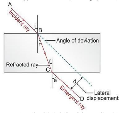
On entering a glass slab, the incident light gets refracted. According to Snell's law, we get
