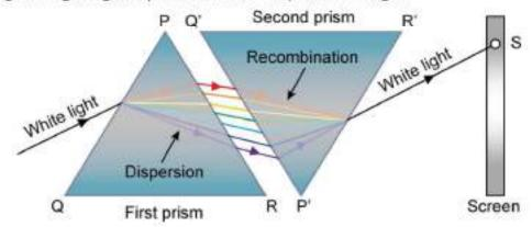
It is essential to place the two identical prisms in an inverted position with respect to each other because the refraction produced by the second prism is equal and opposite to that produced by the first prism.
