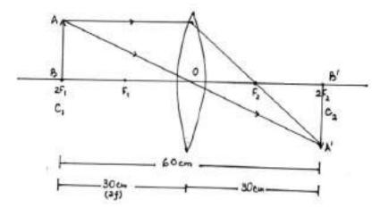
The position of the object is at  $2F_1$  therefore object distance = image distance = 2f
