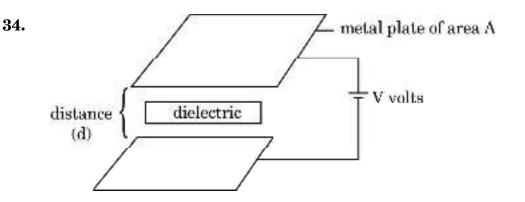
A parallel plate capacitor is an arrangement of two identical metal plates kept parallel, a small distance apart. The capacitance of a capacitor depends on the size and separation of the two plates and also on the dielectric constant of the medium between the plates. Like resistors, capacitors can also be arranged in series or parallel or a combination of both. By virtue of electric field between the plates, charged capacitors store energy.
